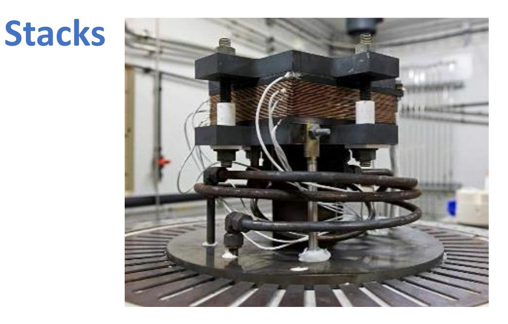
Stack design has been optimized for rSOC operation. A minimization of the internal air pressure drop (by a factor of
